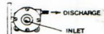
Base vertical on left, discharge points right, on top of pump housing.
